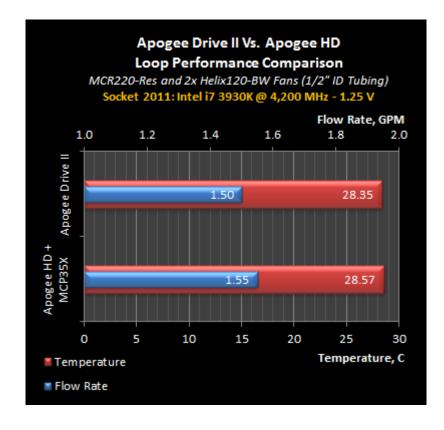
Note: "Temperature Delta" means the difference between the average CPU core temperature and the average air temperature. This reporting method reflects the true efficiency of the cooling system because it eliminates ambient air temperature variations in the data being compared. Users are cautioned that the above data is provided for reference only, and is not directly comparable with CPU temperature values collected a) from an enclosed chassis and b) without deducting ambient air data.
