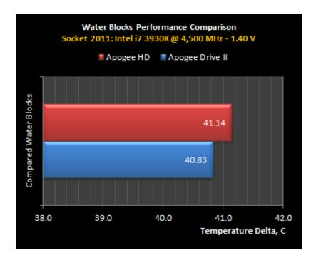
The following chart compares thermal performance of a conventional setup versus one where both water-block and pump have been replaced by an Apogee™ Drive II (1 pump in operations):
