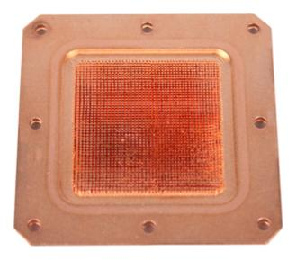
The base-plate is precision-machined from C110 copper. Thermal design of the cooling engine is characterized by Swiftech's fin/pin matrix composed of 225  $\mu m$  (0.009") micro structures.
