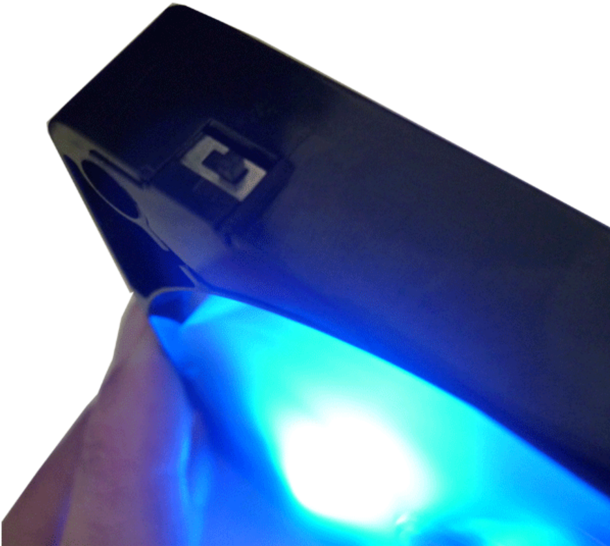
Caption: On/ off Switch for the LED lights mounted on the fan frame
