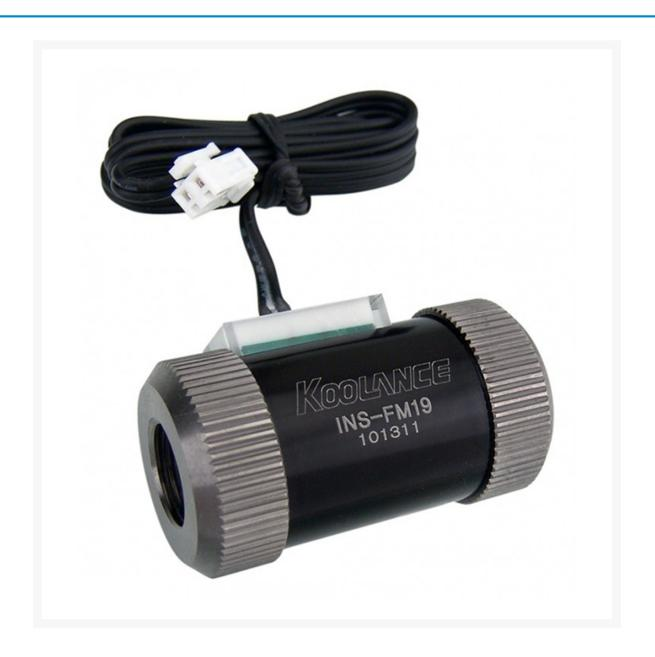
Koolance's inline flow meter provides a visual and electronic indicator of real-time coolant flow rate. Uses G 1/4 BSPP threads. INS-FM19 is electronically identical to INS-FM17N, but has an external metal shell for greater durability.
