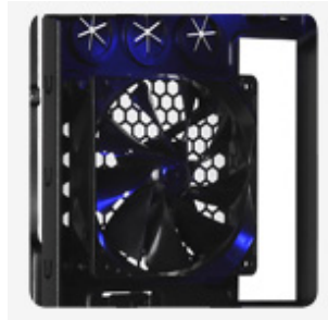
Rear Exhaust 120 mm black fan with Blue LED
