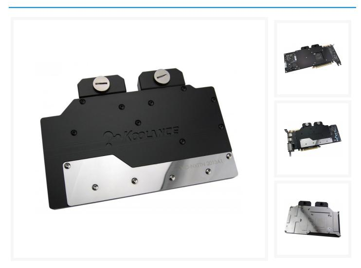
The Koolance VID-NXTTN2 is a full coverage video block for water cooling NVIDIA reference GeForce GTX TITAN, GTX 780, and GTX 780 Ti cards in single and multi video card configurations. It utilizes a high-performance microfin (0.5mm) design made of solid copper with anti-corrosive nickel plating. An aluminum back plate is included to handle the rear memory chips.
