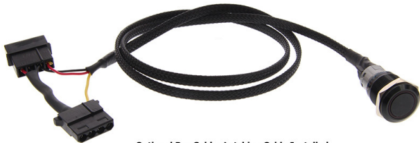
Optional Pro-Solder Latching Cable Installed
