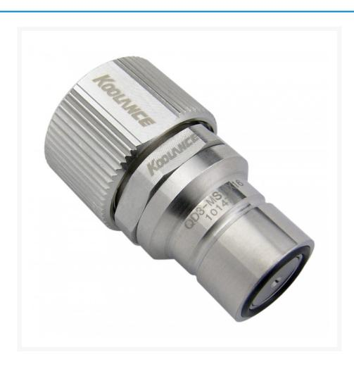
Koolance (patent-pending) quick disconnect no-spill coupling with automatic shutoff. 10mm (3/8") ID, 16mm (5/8") OD male straight connection with compression fitting. It will only fit a Koolance QD3 female quick disconnect.
