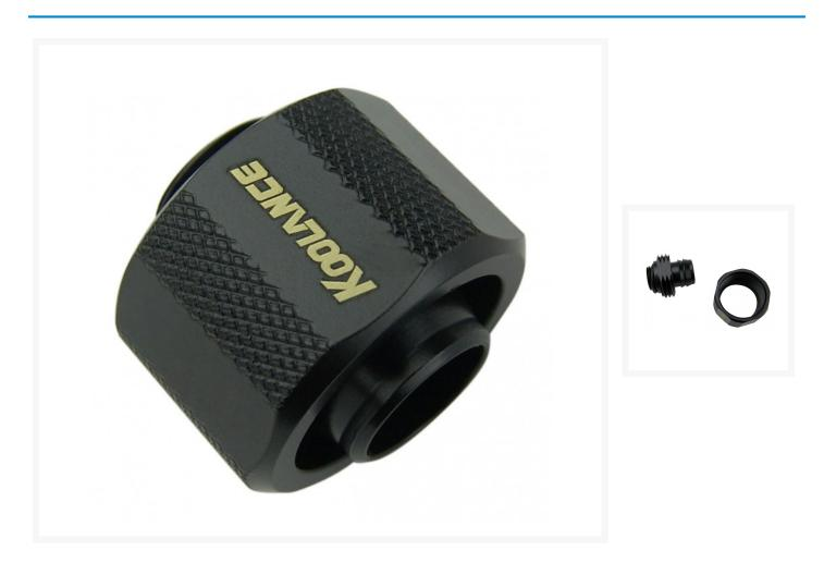
Single fitting for 1/2" (13mm) ID, 3/4" (19mm) OD tubing. G 1/4 BSPP (parallel) thread fitting. Made of brass and includes compression ring.
