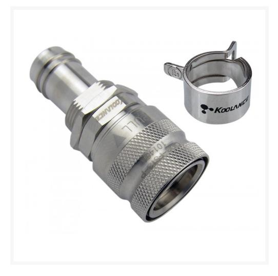
Koolance patented quick disconnect no-spill coupling with automatic shutoff. 13mm (1/2in) ID female panel-mounted hose barb with clamp for 16mm OD (5/8in). It will only fit a Koolance QD3 male quick disconnect.
