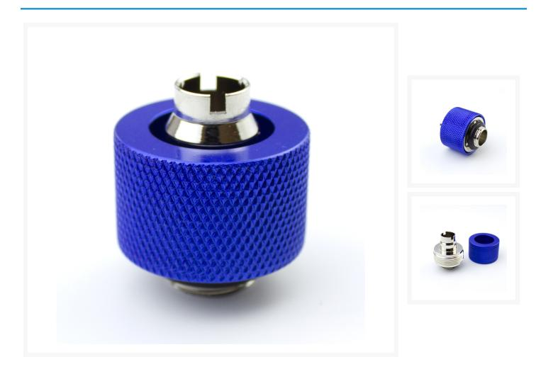
These PrimoChill Ghost Compression Fittings for Flexible tubing are a combination of nickel coated brass inner section with an aluminum ring for tube sealing. The aluminum outside ring makes them light weight and have a knurled texture around the outside to make tightening simple.
