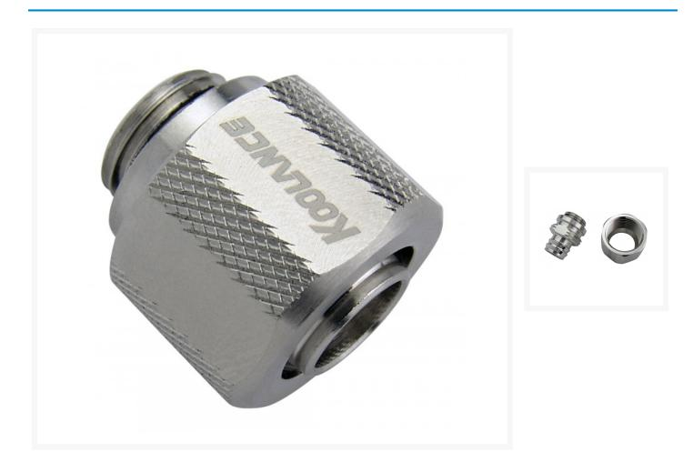
Single fitting for 3/8" (10mm) ID, 1/2" (13mm) OD tubing. G 1/4 BSPP (parallel) thread fitting. Made of brass and includes compression ring.
