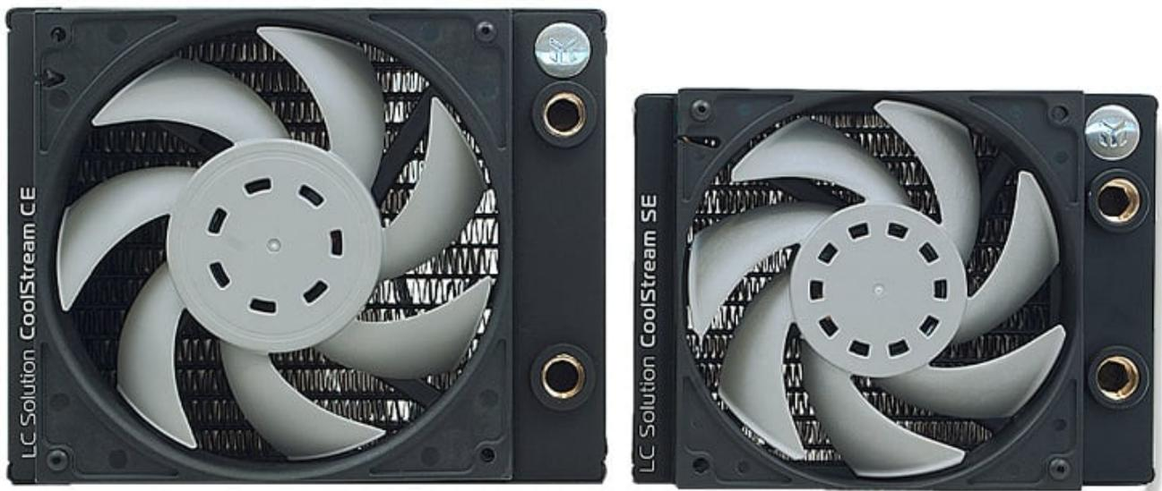
This radiator offers best cooling capacity in the 45mm thick radiator class: Dual stack copper fins provide massive surface area while the parallel flow cooling chambers reduce hydraulic flow resistance to a minimum. Radiator shrouds are tapped with UNC 6-32 threads on both sides to enable push-pull fan installation to even further increase the cooling performance.
