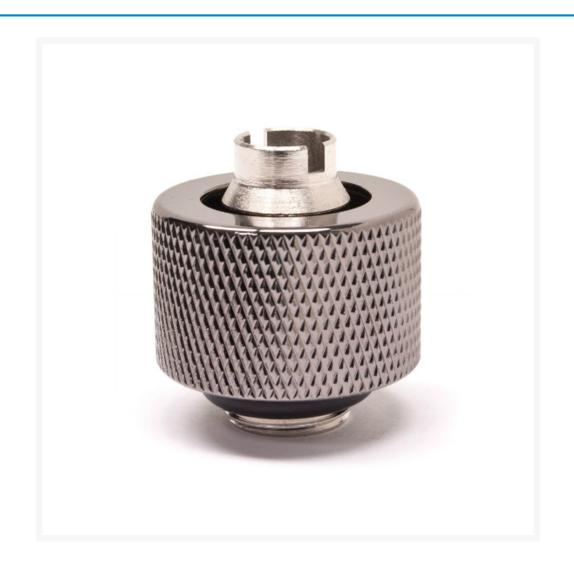
These PrimoChill Ghost Compression Fittings for Flexible tubing are a combination of nickel coated brass inner section with an aluminum ring for tube sealing. The aluminum outside ring makes them light weight and have a knurled texture around the outside to make tightening simple.
