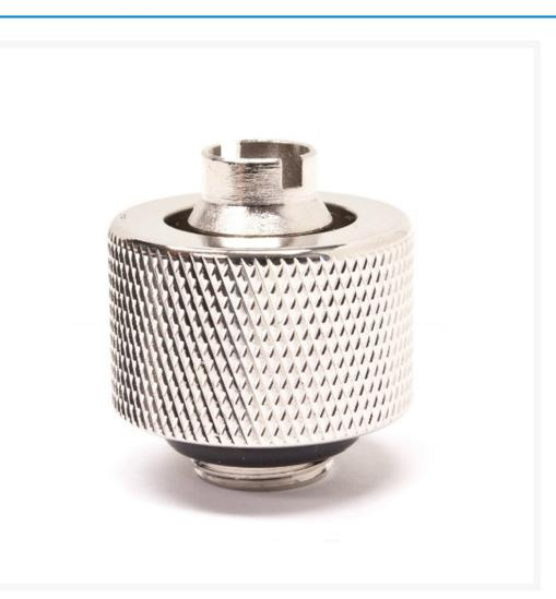
These PrimoChill Ghost Compression Fittings for Flexible tubing are a combination of nickel coated brass inner section with an aluminum ring for tube sealing. The aluminum outside ring makes them light weight and have a knurled texture around the outside to make tightening simple.
