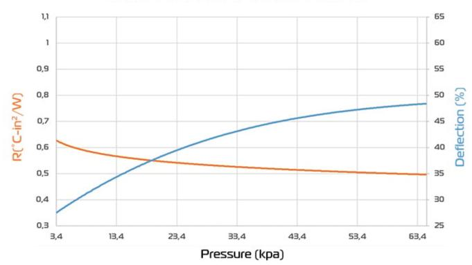
Thermal Resistance vs. Pressure vs. Deflection
