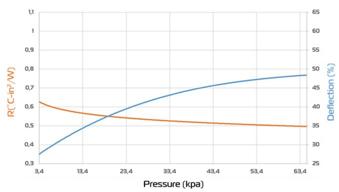
Thermal Resistance vs. Pressure vs. Deflection
