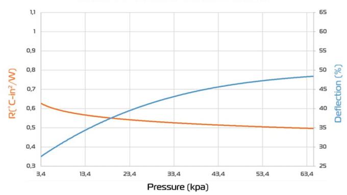
Thermal Resistance vs. Pressure vs. Deflection
