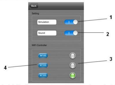
1: Dropped connect again button. When the cellphone use this software, because the lock screen or other reasons result in WIFI can not remote, click this key, if connect successful, then shows
