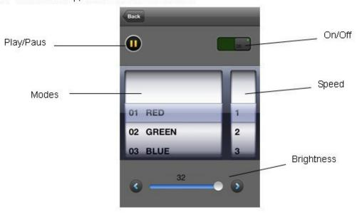
When switch in this state, controller open; When switch in this state, controller off, and at this time it is locked state, unless on/off key, other keys can not use.
