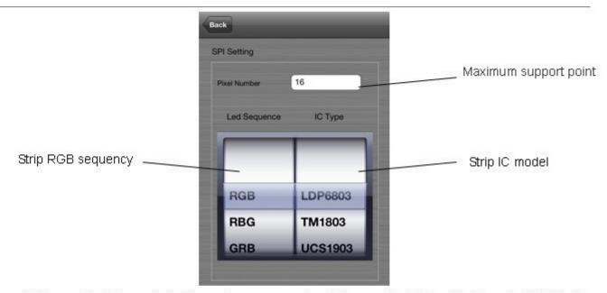
Setting adjustable control strip maximum support point(range 16~1024), strip IC model (10 kinds), strip RGB sequency. Because in the market, many strip the specificate is different, some the sequency is RGB, some is RBG, GRB and so on, so this setting method can suit for all have sequency strip.
