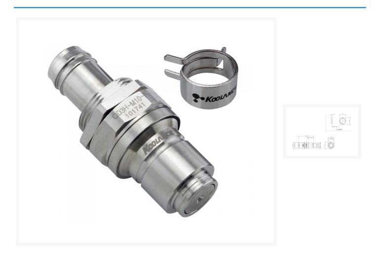
Koolance patented quick disconnect no-spill coupling with automatic shutoff. 10mm (3/8in) ID male panelmountable hose barb with clamp for 13mm (1/2in) OD. It will only fit a Koolance QD3H female quick disconnect.
