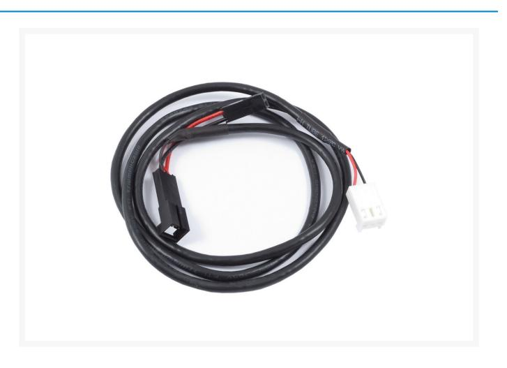
This cable can be used to connect the alarm header of an aquastream ULTIMATE, poweradjust 3 or mps family device with the power switch header of a computer motherboard. This allows for an emergency shutdown of the PC in case of an alarm condition. The cable is to be connected in between motherboard and PC case power switch, the power switch remains operational. Total cable length approx. 70 cm.
