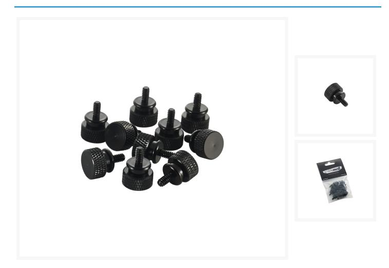
Add another splash of color to your rig with CableMod Anodized Aluminum Thumbscrews. These easy-to-use thumbscrews use a standard UNC 6-32 thread and have a length of 5mm, making them ideal for PC case side panels and PCI slots.
