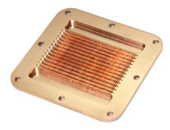
The base-plate is precision-machined from C110 copper. Thermal design of the cooling engine is characterized by Swiftech's fin/pin matrix composed of 225  $\mu$ m (0.009") micro structures; the matrix has been further refined with variable width cross channels to improve flow rate without affecting thermal efficiency.
