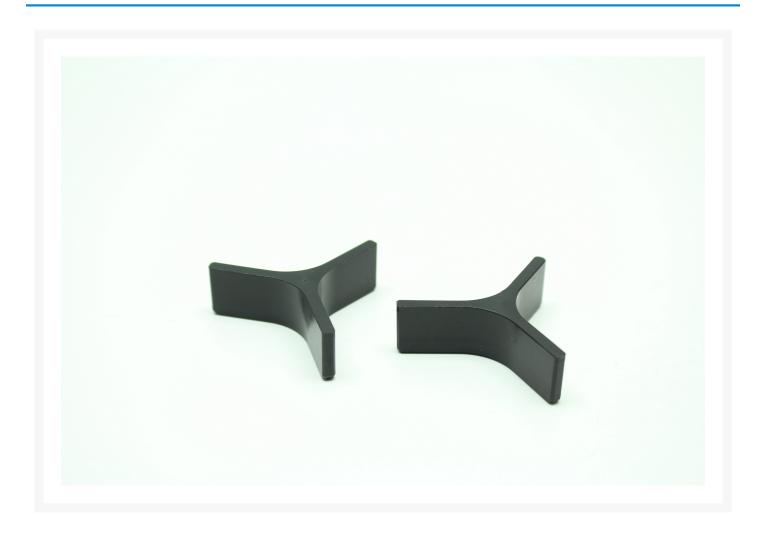
These molded nylon anti-vortex anti-splash Tridents can easily be pressed into any of our MMRS molded end caps or couplers to eliminate or reduce splashing or the formation of a water vortex caused by incoming water entering a flow induced spiral.
