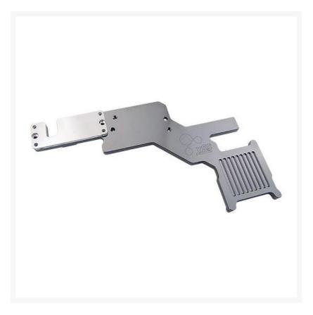
The MB-PLTASR2E targets the northbridge and southbridge chipsets of the ASUS Rampage II Extreme motherboard. As a less expensive alternative to the MB-ASR2E, this heat transfer plate will accommodate a Koolance CHC-120, CHC-122, CHC-125, or MVR-40 water block. (It is not intended to be used alone.) Materials include copper with anti-corrosive nickel plating. G 1/4 nozzle threading.
