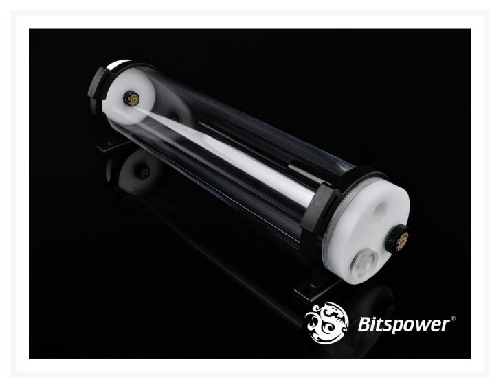
High quality multi option compensating reservoir for most advanced users! Manufactured of first class quality acrylic tube. Bottom part gives user 3 options for placing the G1/4" fittings/barbs as inlet or outlet. Top with G1/4" thread is can be used for additional fitting/barb as inlet of filling port. The compensating reservoir is very easy to fill and is sealed with high quality rubber gasket.
