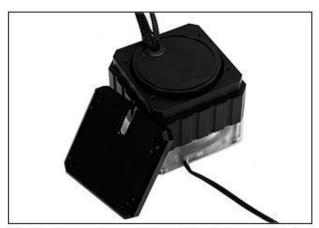
3.In the figure, the radiator refit kit piece only plays a decorative role. For example, if the D5 pump is used, and the adjustment is required, only the radiator refit kit piece can be removed to adjust the speed without affecting the normal use
