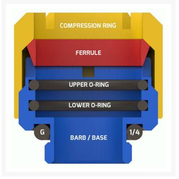
Designed as the second generation of Monsoon's popular line of Economy Fittings, EV2 features significant improvements in multiple areas including substantial improvements in resistance to tube pull out, reductions in tube wobble, and dual O-ring seals for improved leak prevention.
