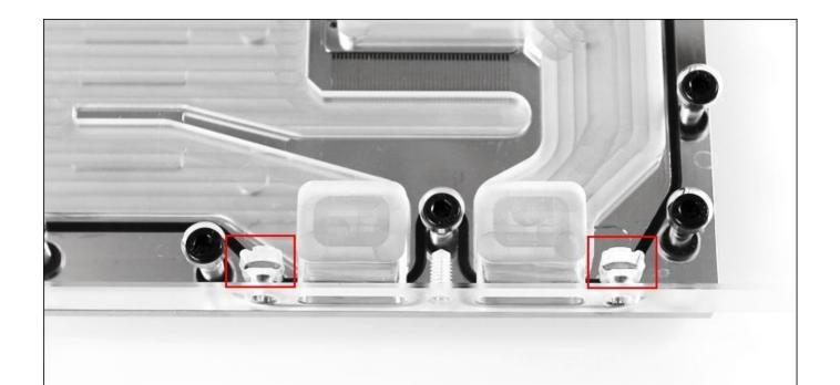
Pay attention to the two square nuts in the location of the red mark, so as to avoid falling off and affect the installation.
