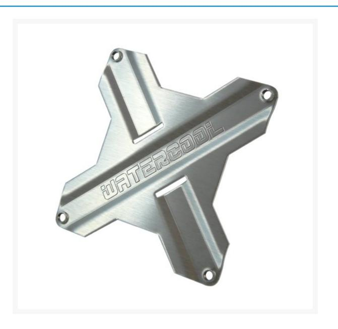
Universal backplate to be used with socket 1366. Integrated M4 threads in the backplate allow screws and stand-offs to be screwed in directly. The HEATKILLER® CPU Rev3.0 series includes the necessary mounting material. For use with Rev 2.6 or lower, screws of increased length are required.
