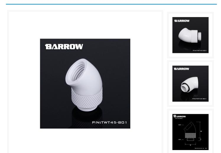
The Barrow G1/4" Thread 45-Degree Rotary Fitting Adapter allows you to extend your fitting port at a 45 degree angle, allowing larger fittings to be used or allowing connection of other fittings! A great solution for people not using tubing between very close blocks! These have a rotary connection allowing the adapter to spin 360 degrees. This keeps tubing from kinking or breaking.
