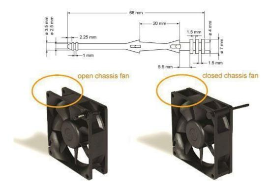
Note: These fan mounts work only on fans whose mounting holes are the easy fan mount type (which have no additional plastic beyond the hole).
