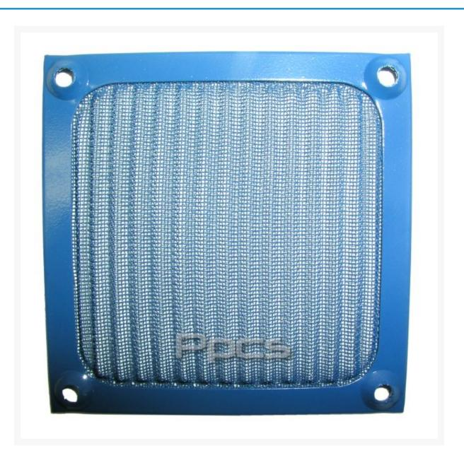
Aluminum fan guard with filter. This filter has an efficient thin design that effectively stops dust from entering the case, while minimising airflow restriction. 120mm in size. The tightly woven aluminum corrugated mesh screen is encased in a formed aluminum frame built for ruggedness and durability.
