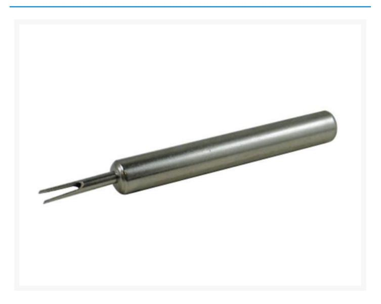
For removing ATX pins (ATX20pin / ATX24pin) & P4-12V 4pins from the the connectors. Without a pin remover, you would have to cut off the wires and re-solder the pins to change the connectors. With the Toolx<sup>™</sup> Pin Remover, you can just remove the pins with the wire and re insert them into the new connectors.
