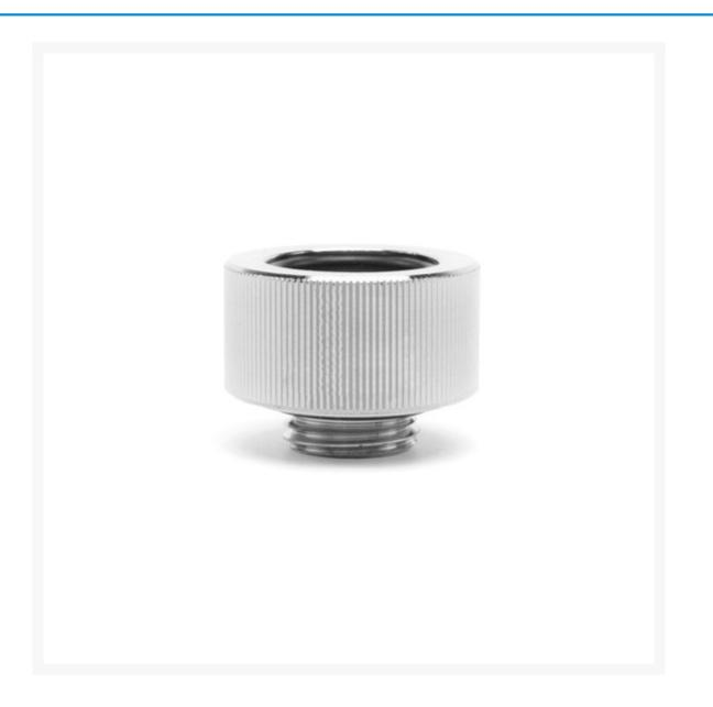
EK-HTC Classic 14 (*Hard Tubing Compression*) Fittings are 14mm hard-tube compression fittings designed for use with solid tubing such as Acrylic and PETG. With a high-quality finish, the EK-HTC Classic Fittings are an aesthetically appealing and secure option for your custom loop liquid cooling system. A non-intrusive, minimalistic look, with NO added branding at all.
