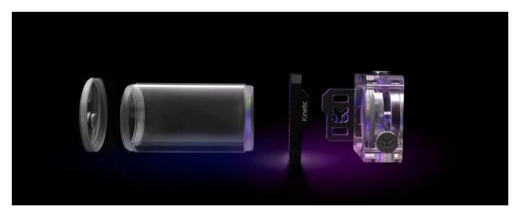
Another three industry-standard G1/4" ports are available in the bottom combo housing which is also made of CNC machined cast acrylic. Aside from the in and out ports, it features a side port usable as either an optional inlet or a drain port. Mounting is done through 4 pillars on the bottom of the pump-reservoir combo unit. The addressable LEDs are placed in a ring directed toward the coolant. Any unwanted hot-spots of the D-RGB LED of the combo unit is covered by a CNC machined aluminum piece.
