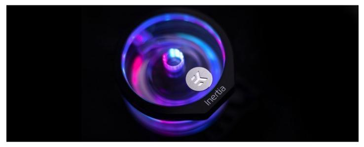
The top is made of quality CNC-machined cast acrylic material with a black ring to cover the LED hotspots as the proper LED implementation is one of the main focus points of EK.
