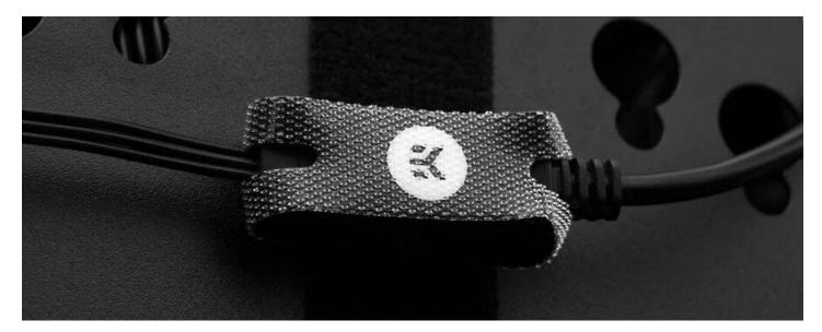
Also, there is another self-adhesive strap that is intended to be stuck to the backside of the motherboard tray, and it grabs the main part of the fastener and holds it in place of your choosing. These two together create the cable management system called EK-Loop CMS.
