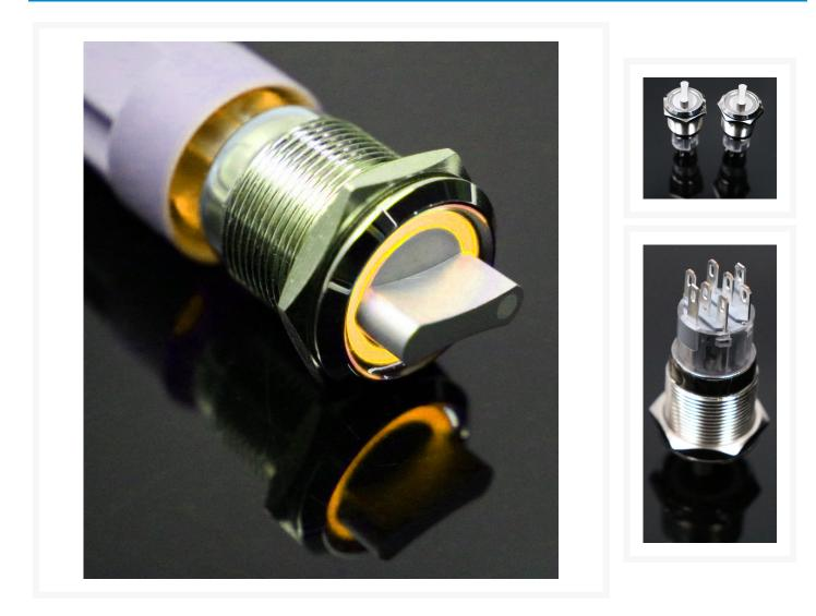
These switches are to be installed in a 19mm diameter slot and have 3 different positions when turning dial. They are powered by 12V and are made of stainless steel. They also have a illuminated Ring around the top.
