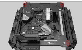
8. It is necessary to install the screws marked in red in the drawing to fix the radiator enhancement kit with the case.
