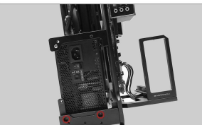
7. It is necessary to install the screws marked in red in the drawing (use the screws for power adapter block) and connect the 90-degree power extension cable.
