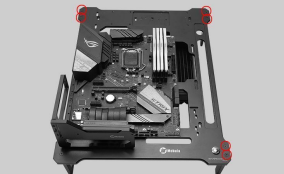
5. It is necessary to remove the screws marked in red in the drawing and remove the support of the case.
