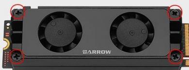
5.Install the red position screws in the picture, the installation is complete
