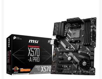
The MSI X570-A PRO AM4 ATX Motherboard is built on the AMD X570 chipset, supporting second- and thirdgeneration AMD Ryzen processors with an AM4 socket. It has four memory slots for up to 128GB of dualchannel DDR4 RAM, which can be overclocked to up to 4400 MHz. For storage, it's equipped with six SATA III ports and two M.2 slots.
