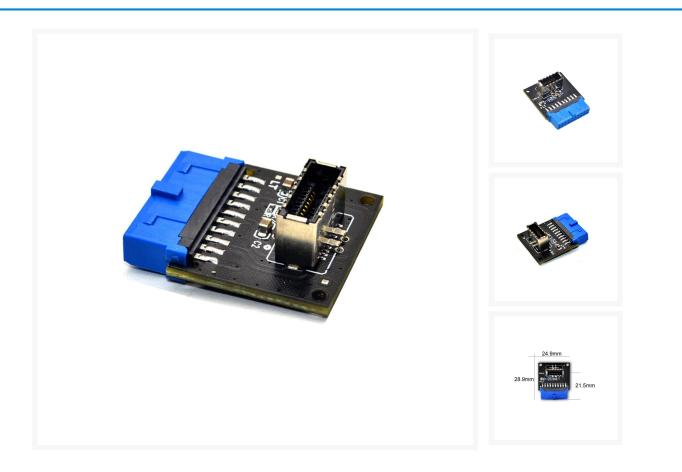
This is a front panel USB Type C Gen 3.1 to USB 3.0 front panel connector.
