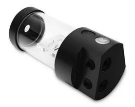
The reservoir comes with a pre-installed anti-vortex insert and the capacity of the EK-RES X3 250 D-RGB variant is around 440ml of liquid. The package also includes a polyether anti-cyclone foam to optionally replace the acrylic anti-vortex insert.
