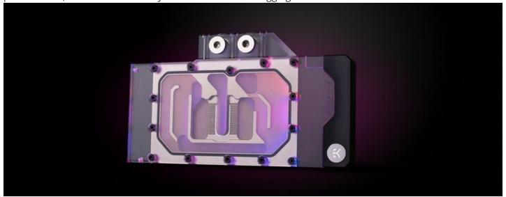
The base of the block is CNC-machined out of nickel-plated electrolytic copper, while its top is CNC-machined out of glass-like cast Acrylic. These 2nd generation Vector GPU water blocks also feature plexi terminals that match the top cover. The watertight sealing is ensured by high-quality EPDM O-rings, while brass standoffs are already pre-installed and allow for a safe and easy installation procedure.
