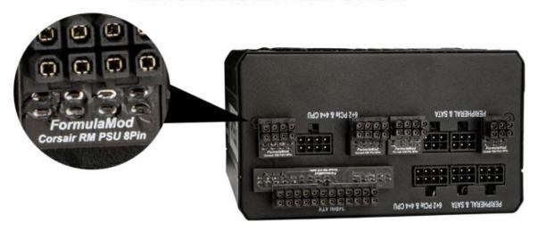
Please note that the sockets on both sides are marked with text, and PSU stands for the socket that is inserted into the PSU direction. Take the above picture as an example, the PSU 8Pin should be connected to the PSU instead of being exposed and waiting for the cable to be connected.
