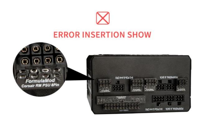
Please note that the sockets on both sides are marked with text, and PSU stands for the socket that is inserted into the PSU direction. Take the above picture as an example, the PSU 8Pin should be connected to the PSU instead of being exposed and waiting for the cable to be connected.
