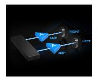
The Sound BlasterX AE-5 is the first sound card to feature Xamp, our custom-designed discrete headphone amplifier. Each audio channel is individually amplified, allowing the AE-5 to deliver a whole new level of pristine audio fidelity in an unaltered lossless model to each earcup regardless of demand.
