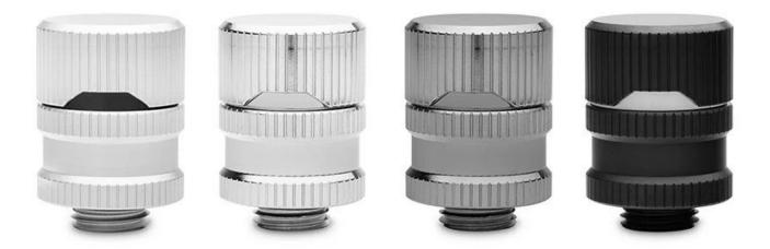
This drain valve has an advantage over the traditional ball valves in terms of size. It has a smaller footprint, secure locking, and an easy open/close mechanism that works on a slide. It has a male thread on one end, allowing you to screw it directly into a G1/4" female port on any water cooling component without the use of an adapter fitting as traditional ball valves do.
