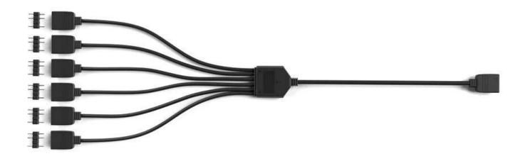
It features standard 3-pin D-RGB headers and the male-male connector pins are also included in the packaging. The splitter cable can be used with any standard 3-pin 5V D-RGB controller or any of the popular RGB sync technologies from all major motherboard manufacturers. The arrow marking on the 3-pin LED connector is to be aligned with the +5V marking on the D-RGB (addressable) header.
